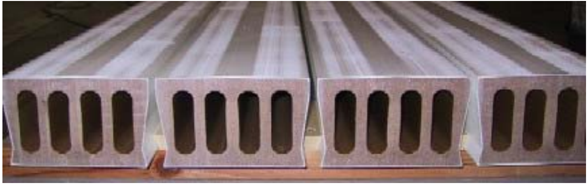
Figure 2.1 Ribbed Box Sections Composed of a Wood-poly (vinyl chloride) Composite Developed by Washington State University for Pier Decking for the US Navy.
