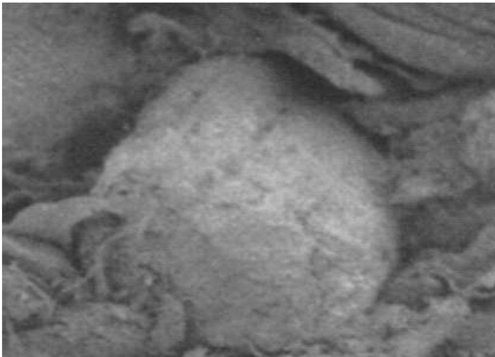
Fig. 4.5: Microscopic images showing particle matrix interface on the fracture surface of a dry (top) and saturated in seawater (bottom) flat pressed coupon.
